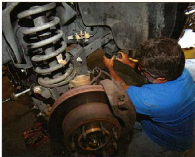
Mark Lankhorst and his friend Keith Spriggs lifted the Dodge on a hoist at KC Customs and tore into the truck Saturday morning. Lankhorst and Spriggs supported the AAM 9 1/4-inch front axle on jack stands and unbolted the factory coils and suspension links.
