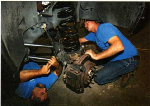
Spriggs and Lankhorst then lowered the front axle as far as it would go and removed the original front coil springs and shocks. The new Trailmaster coil springs and front shocks were installed and the Trailmaster suspension links were bolted in one at a time.
