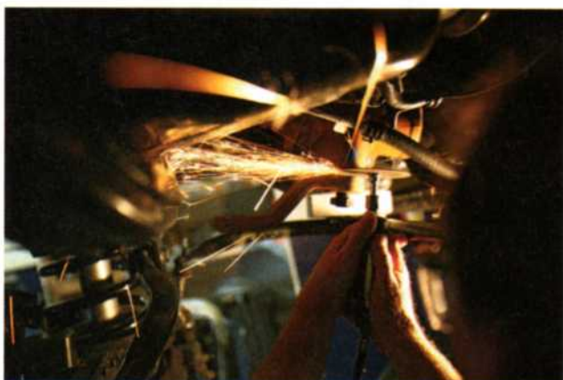
He figured cutting the arm off could damage the steering shaft, heating it might ruin the steering box's seal, and he broke the only puller Snap-On sells that would fit in the small gap. The solution was to use a thin cut-off wheel to grind away the top of the factory arm until there was enough room to fit the pitman arm puller.
