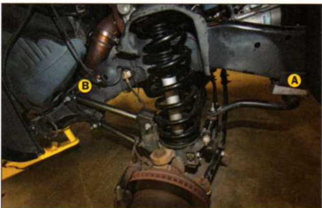
The Trailmaster kit used two solid pieces of 6061 aluminum to lower the stock sway bar mounts (A), and the factory brake lines were reused after their attachment points were modified. The only real challenge was the top suspension link bolt (B). When Dodge assembles the suspension at the factory, there's no engine or exhaust in the truck. In order to remove the bolt, you have to cut the head off, and pull it out. Trailmaster provided a new bolt in the kit, but the 6.7L's exhaust was so large that Lankhorst couldn't fit a sawzall blade in there to make the cut. He decided to unbolt the exhaust at the turbo, lowered it out of the way, and reused the factory bolt to attach the Trailmaster suspension link.
