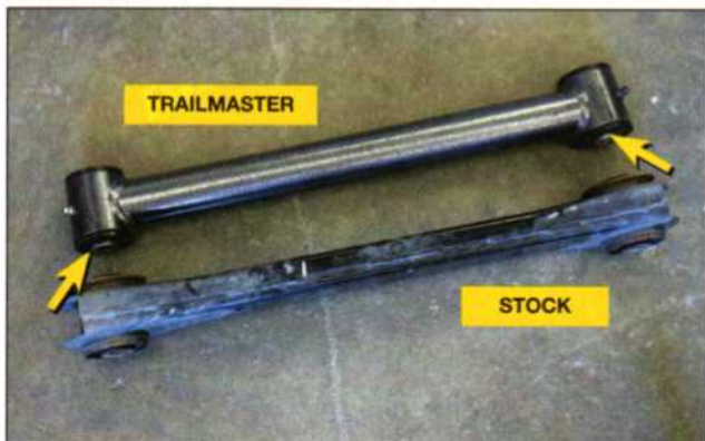
The new Trailmaster 4-inch lift kit came with longer tubular steel suspension links and urethane bushing that had to be installed. Lankhorst found that the steel sleeves that pressed into the bushings (arrow) were too wide to fit into the brackets on the axle, so Spriggs took them to a local machine shop to have them narrowed.
